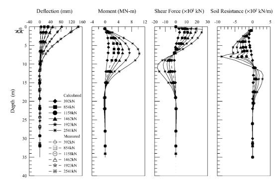
Fig. 9. Analyzed results on laterally loaded drilled-shaft.
