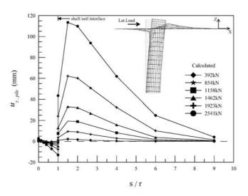
Fig. 14. Upward movement of ground soil in front of the laterally loaded shaft.
