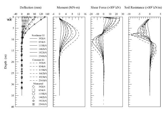
Fig. 10. Comparisons of analyzed results on laterally loaded drilled-shaft.
