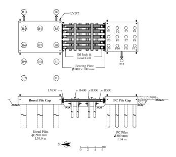
Fig. 4. Layout of laterally loaded piles test [2].
