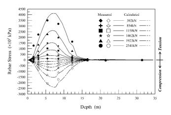
Fig. 13. Stress distribution of rebar along the shaft.
