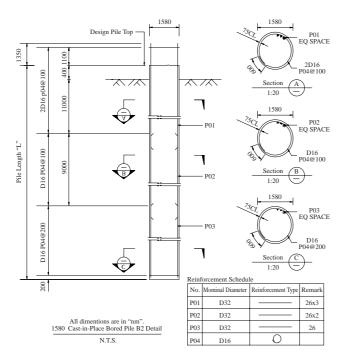
Fig. 5. Details of cast-in-place drilled shaft for B2 [2].
