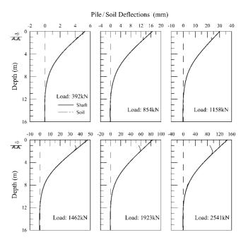
Fig. 15. Separated state between shaft and rear soil under different loading levels.
