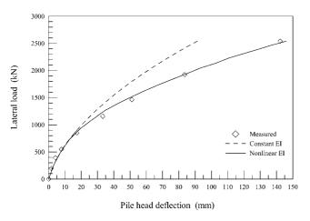
Fig. 7. Displacement of pile head under lateral load.
