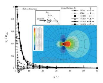
Fig. 8. Variant displacement of ground surface under different loading levels.
