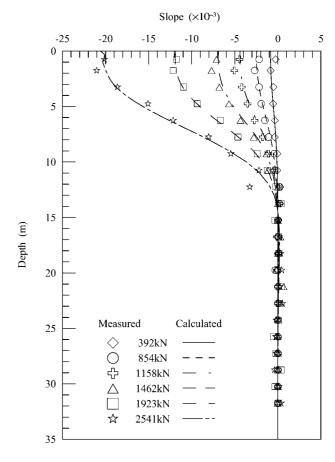
Fig. 11. Variation of slope along the shaft.
