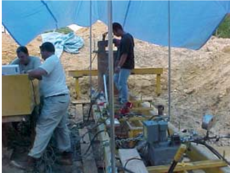
Figure 51. Loading Frame and Instrumentation Set-up
