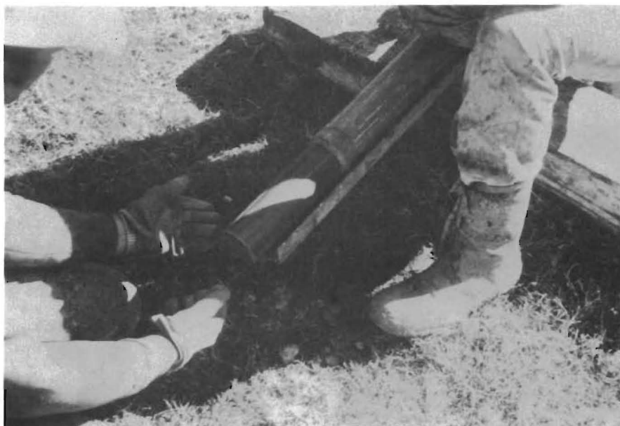
Fig 4.7. Soil sample partially pushed out of the push barrel.
